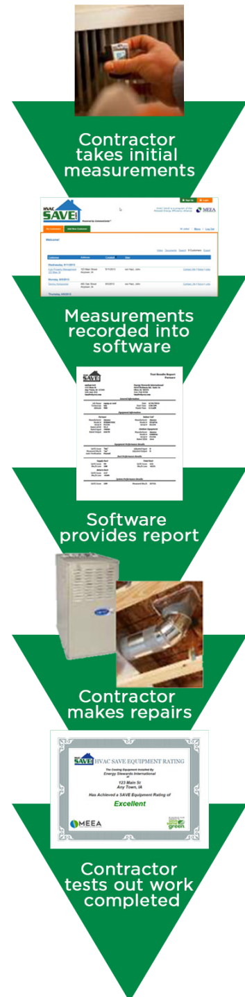
Figure 1: The HVAC SAVE Process and Workflow
