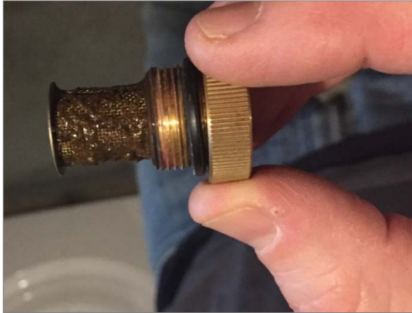
Figure 19. Clogged Filter at Portland Site
