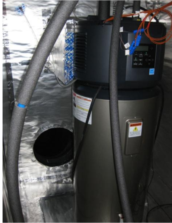
Figure 3. GeoSpring Installed in Test Chamber
