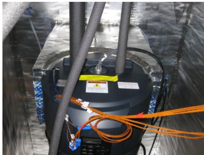
Figure 4. GeoSpring Instrumentation Top View
