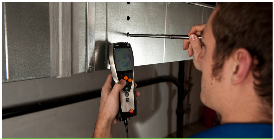
HVAC SAVE Certified Contractor Measuring Airflow Photo courtesy of the Midwest Energy Efficiency Alliance (MEEA)
